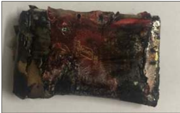
Fig 2- Image of blasted mobile phone battery, brought by the attendant.
